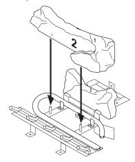
Figure 46 - Installing Log No. 2
